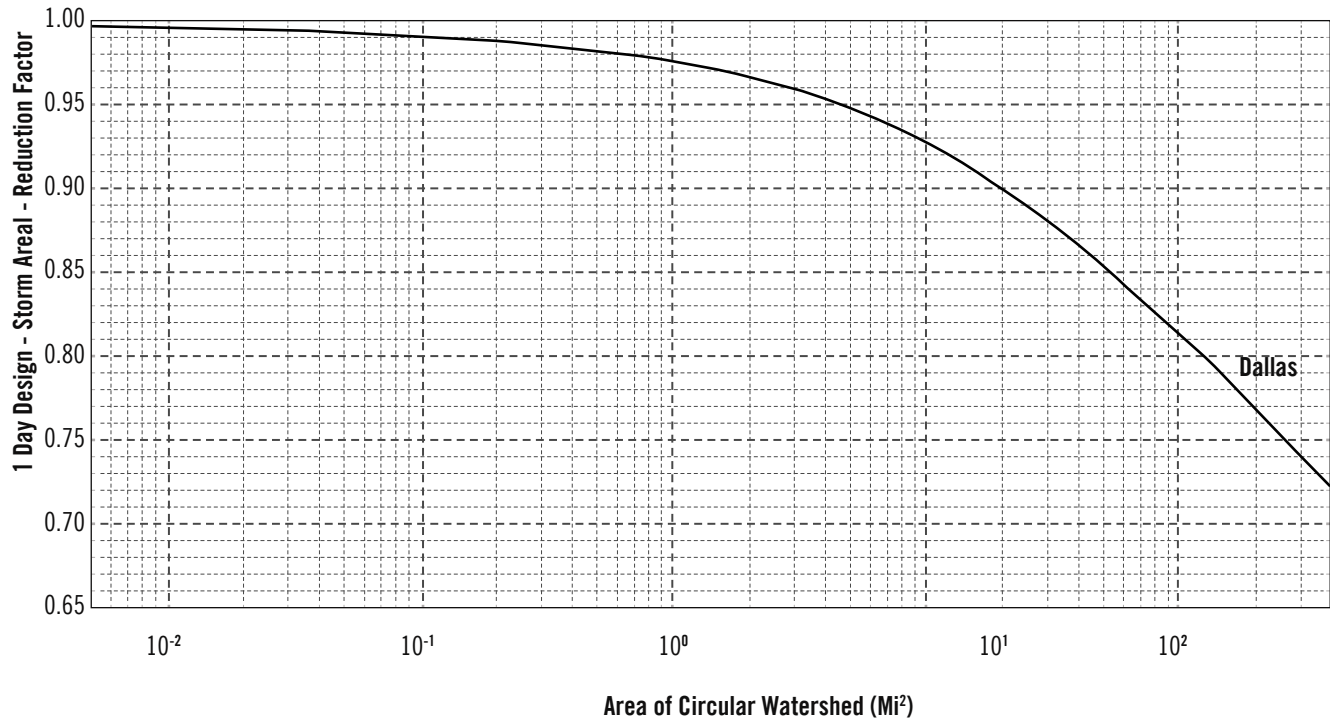
Figure 2.2 Areal Reduction Factors for Small Watersheds for 50% AEP or Greater 1-day Design Storms
